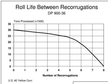
Larger diameter rolls will process more tons before recorrugation, and will have a deeper roll chill or hard working surface. Because of the better nip angle, large diameter rolls are often used in flaking operations where roll corrugations may be very fine to prevent cutting the grain while making thin, uniform flakes. Larger diameter rolls must also be used in machines with longer rolls to maintain the degree of stiffness required for holding the rolls in position.
