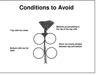
the possibility exists that material may begin to "pile up" in the nip. This condition must absolutely be avoided since the grain slipping in the roll nip will cause greatly accelerated roll wear.
